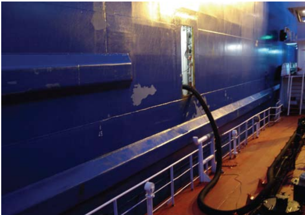
Oil Bunkering (Example)
