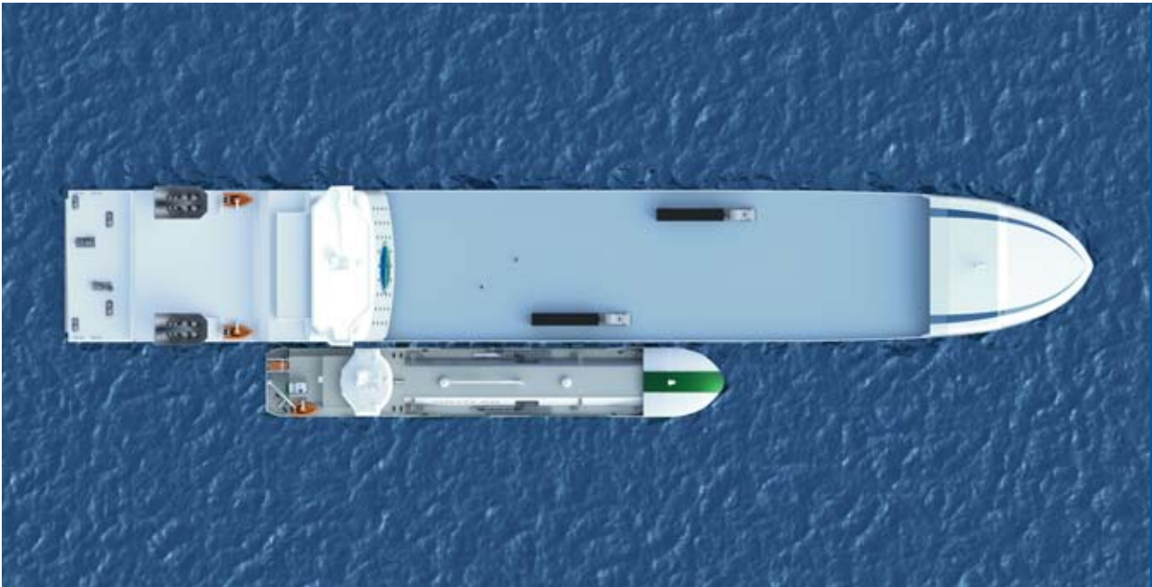
Fig.1 - Typical Bunkering Mooring Arrangement
